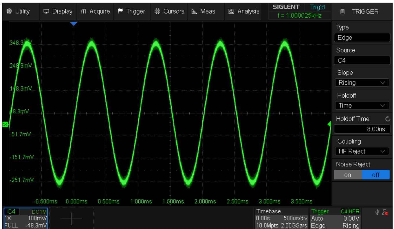
Fig. 74 SDS824X\_HD\_Trig\_Noise\_HFRJ
