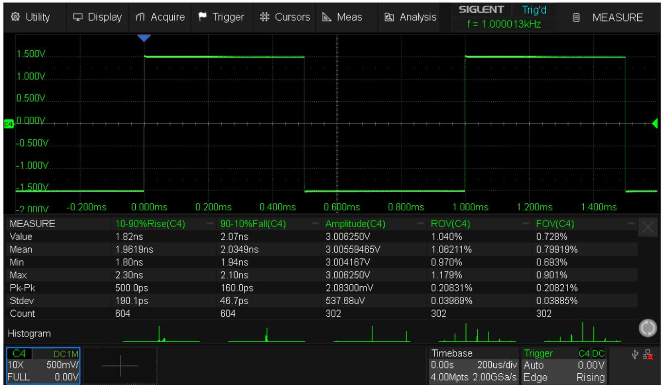
Fig. 133 SDS824X\_HD\_Probe\_PP510\_PR\_1kHz
