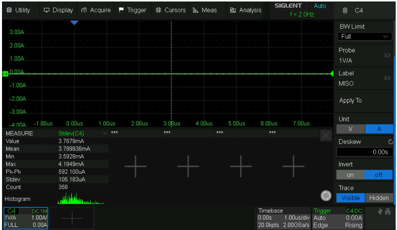
Fig. 144 SDS824X HD\_Ch\_Current\_1V\_A
