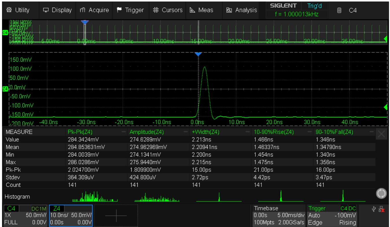
Fig. 15 SDS824X\_HD\_Pulse\_W2ns\_RT500ps\_2GSa\_Norm\_Zoom
