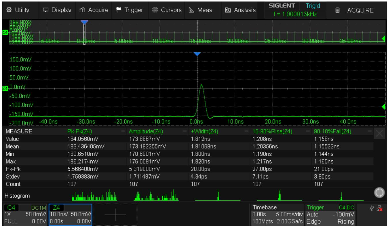
Fig. 18 SDS824X\_HD\_Pulse\_W1ns\_RT500ps\_2GSa\_Norm\_Zoom
