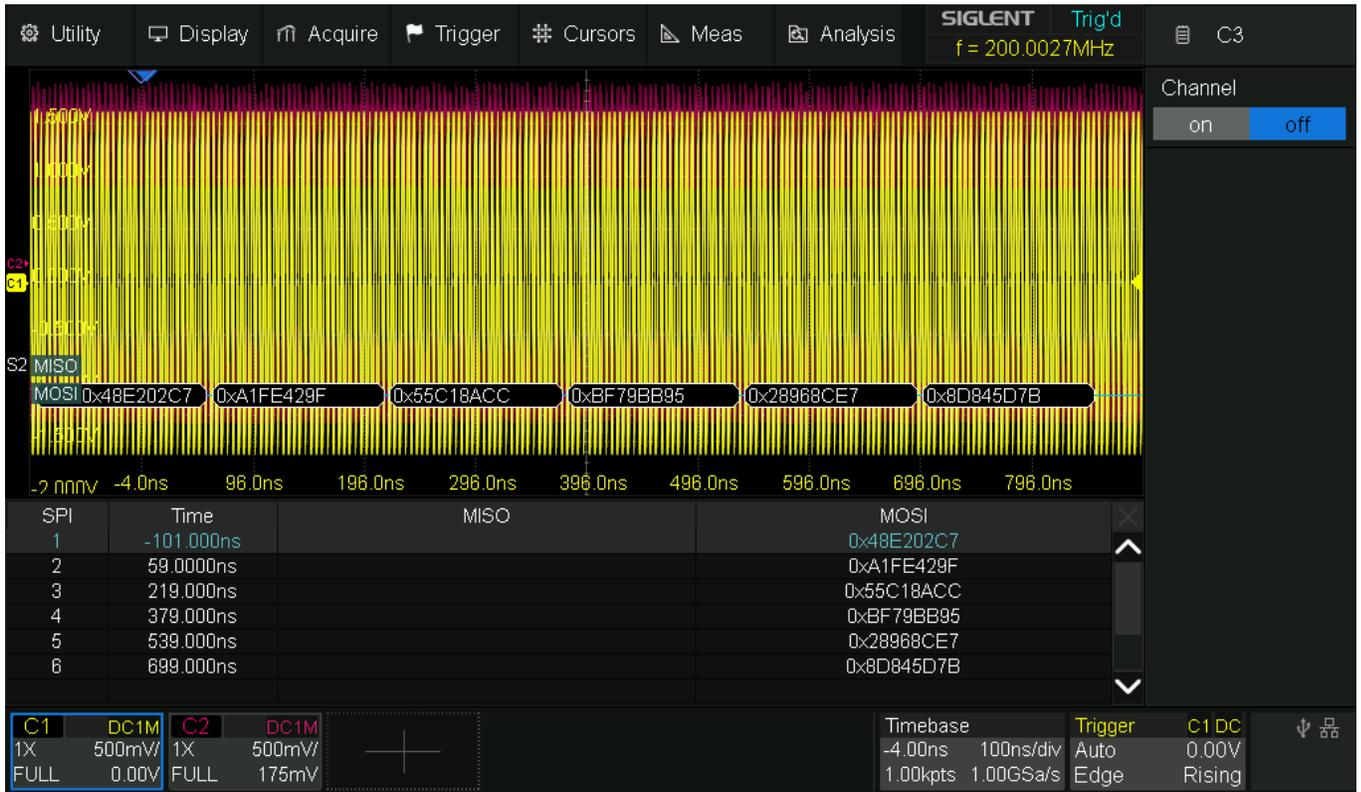
Fig. 125 SDS824X\_HD\_SPI\_200Mbps\_2Ch
