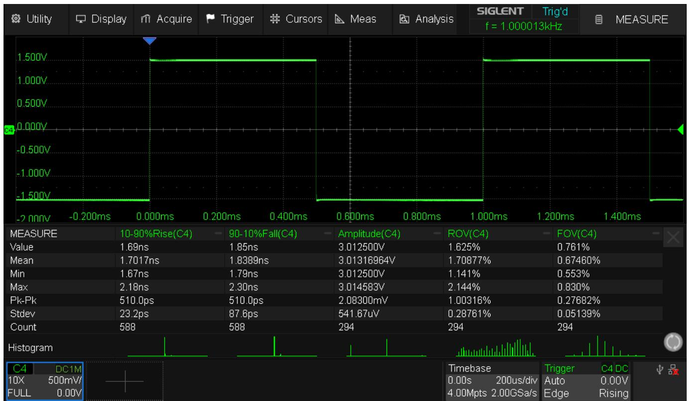
Fig. 142 SDS824X\_HD\_Probe\_PP5050A\_PR\_1kHz
