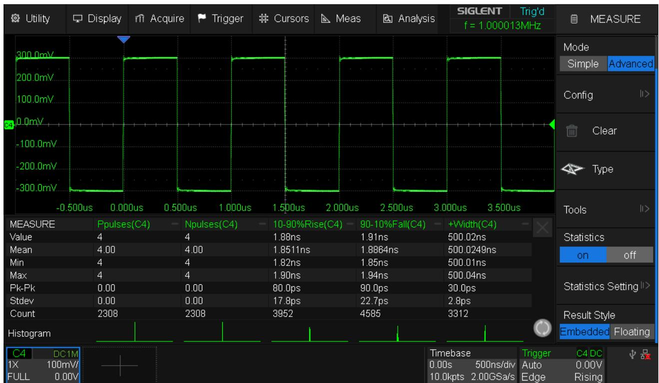
Fig. 78 SDS824X\_HD\_Measure\_Advanced\_Embedded
