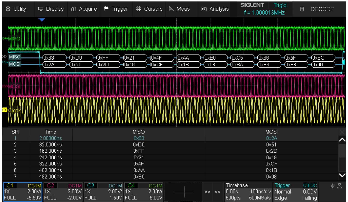
Fig. 119 SDS824X\_HD\_SPI\_100Mbps
