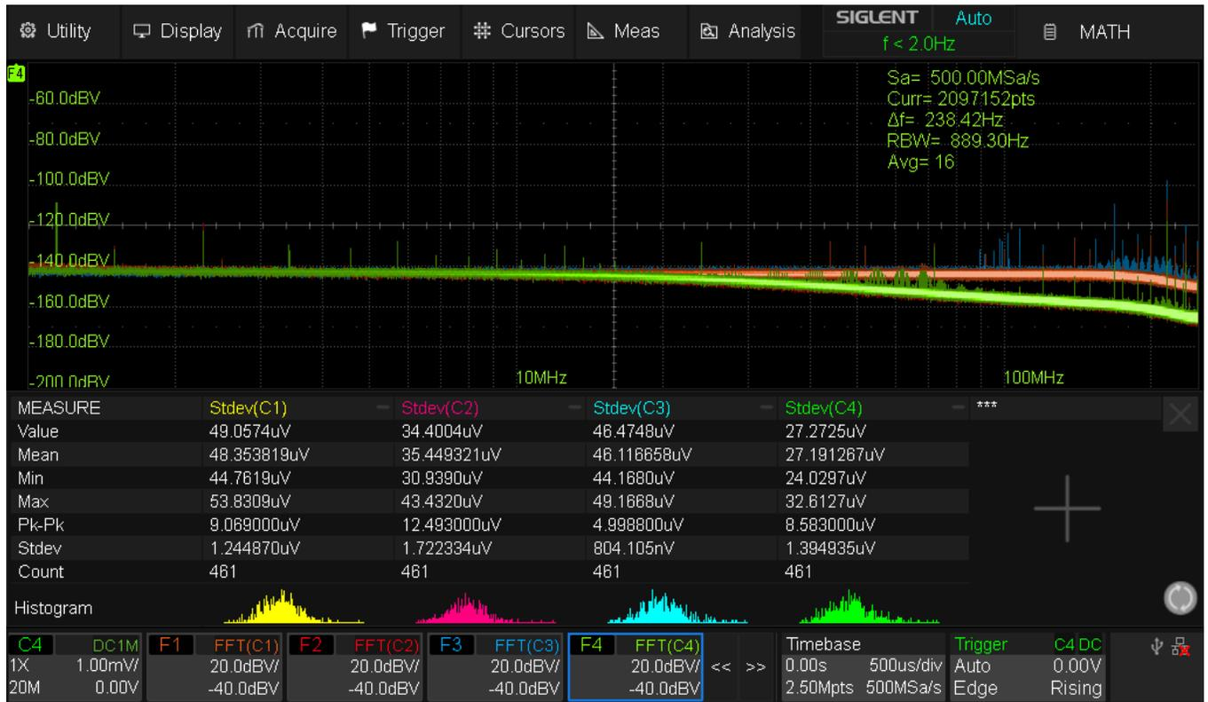
Fig. 32 SDS824X\_HD\_Noise\_200Hz-200MHz\_4Ch
