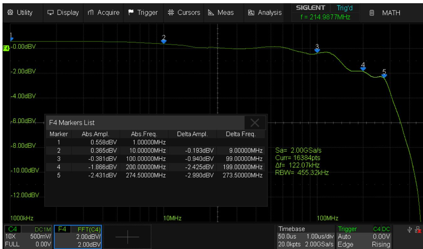
Fig. 132 SDS824X\_HD\_Probe\_PP510\_FR
