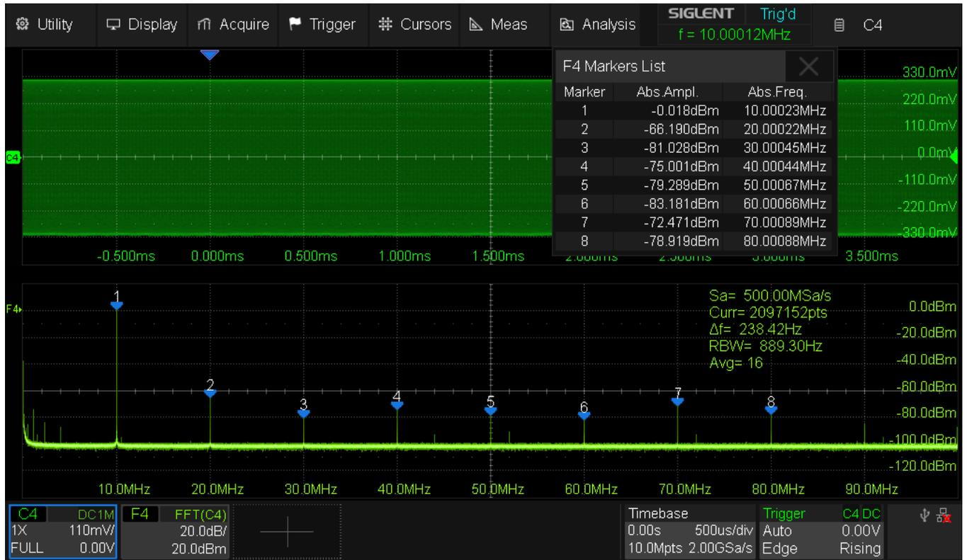
Fig. 109 SDS824X\_HD\_FFT\_THD\_10MHz
