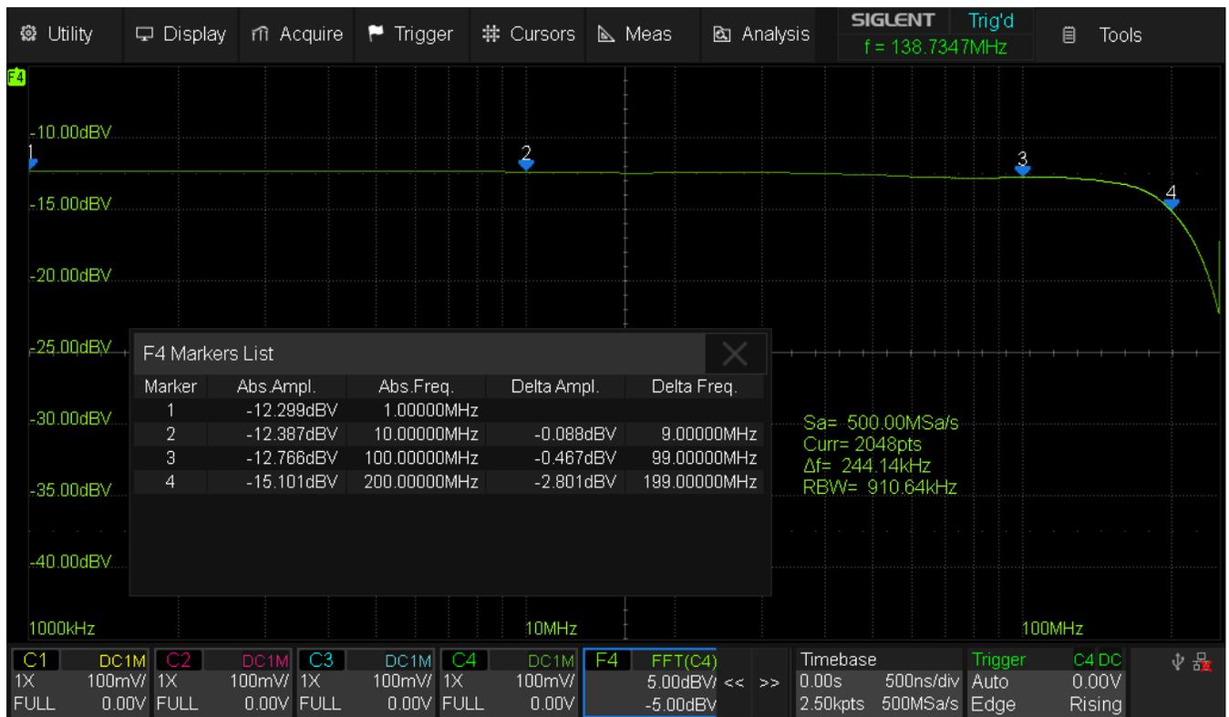
Fig. 3 SDS824X\_HD\_FR\_500MSa\_log
