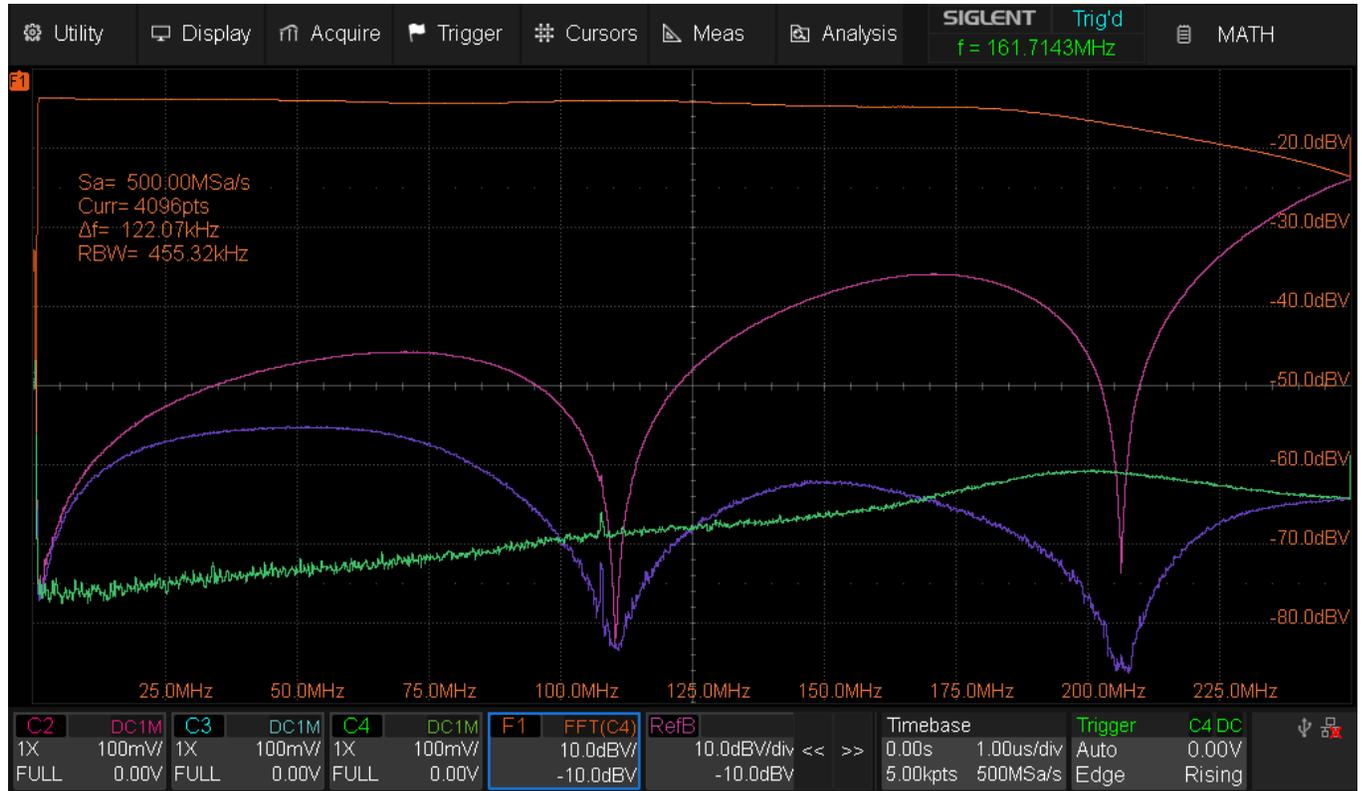
Fig. 28 SDS824X\_HD\_Aliasing\_500MSa
