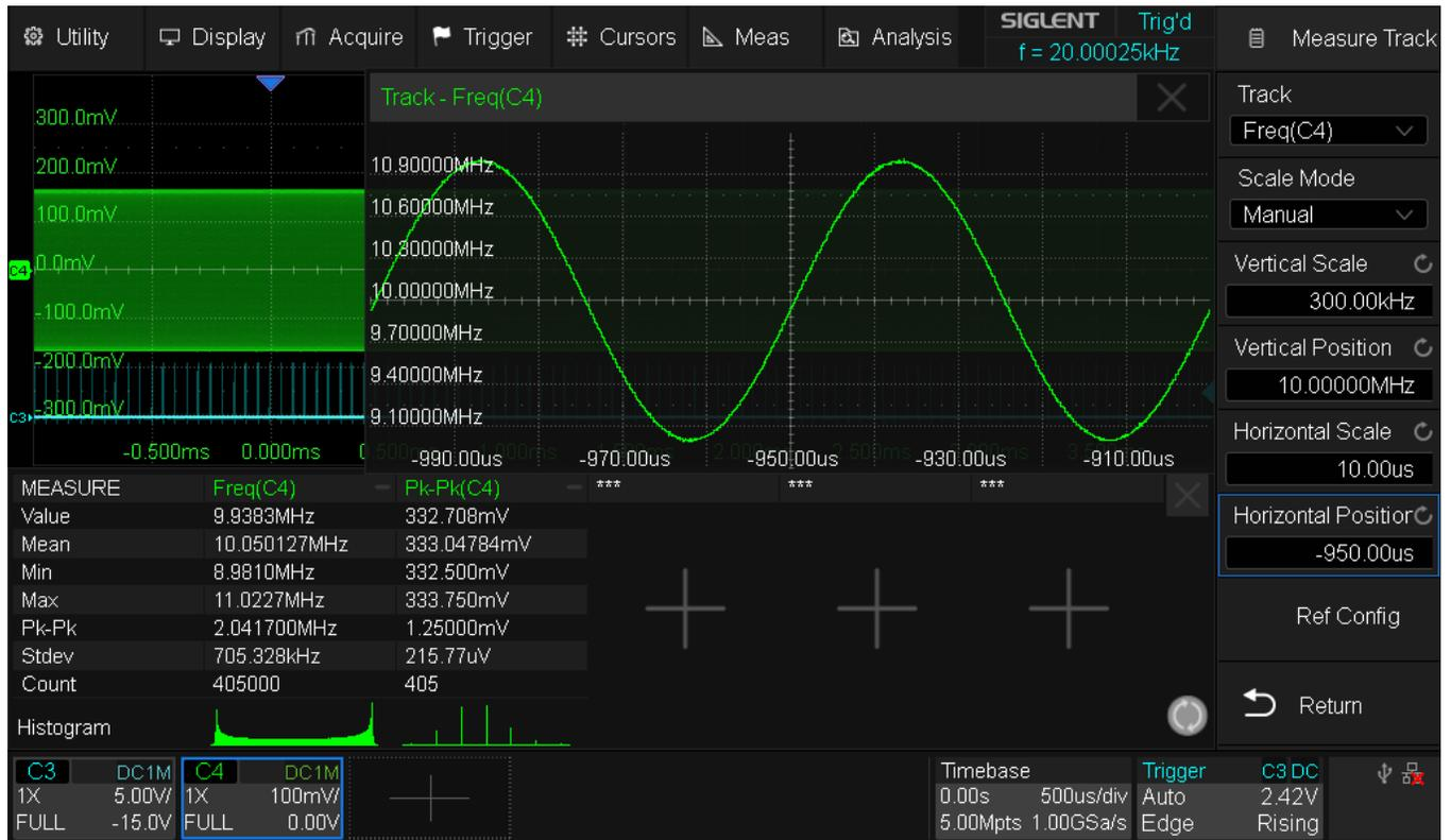
Fig. 89 SDS824X\_HD\_Measure\_Track\_FM
