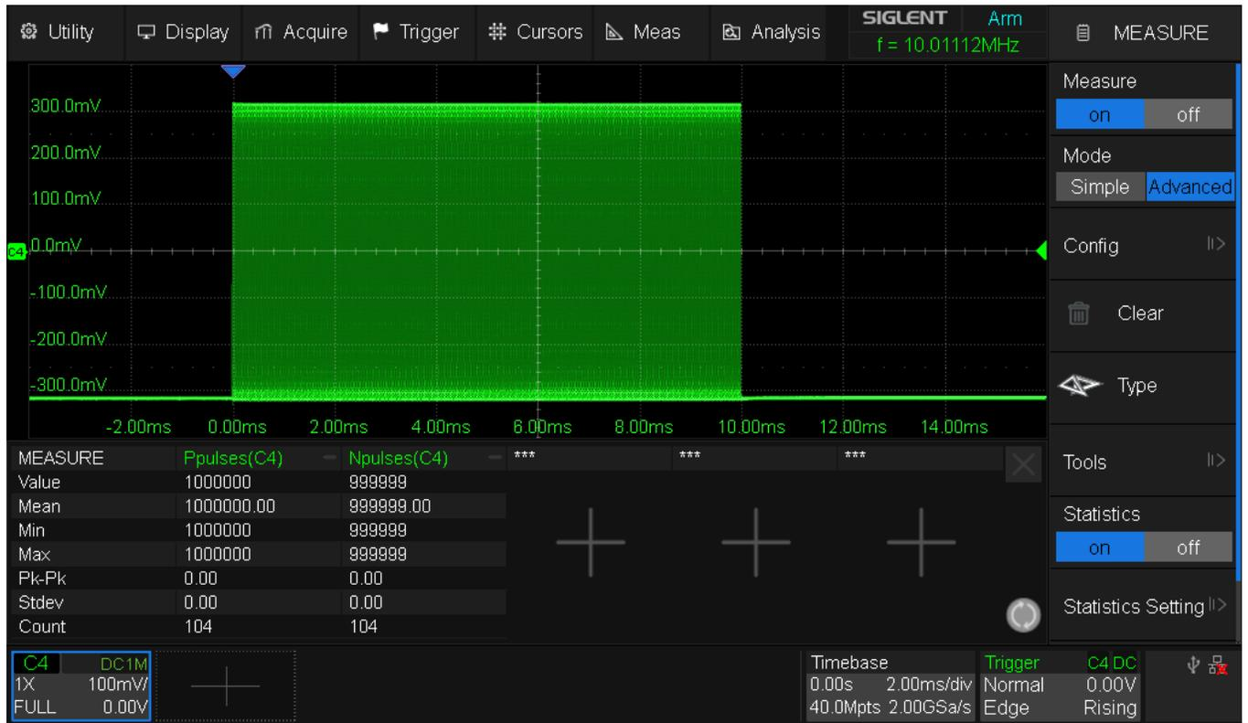
Fig. 90 SDS824X\_HD\_Pulsecount
