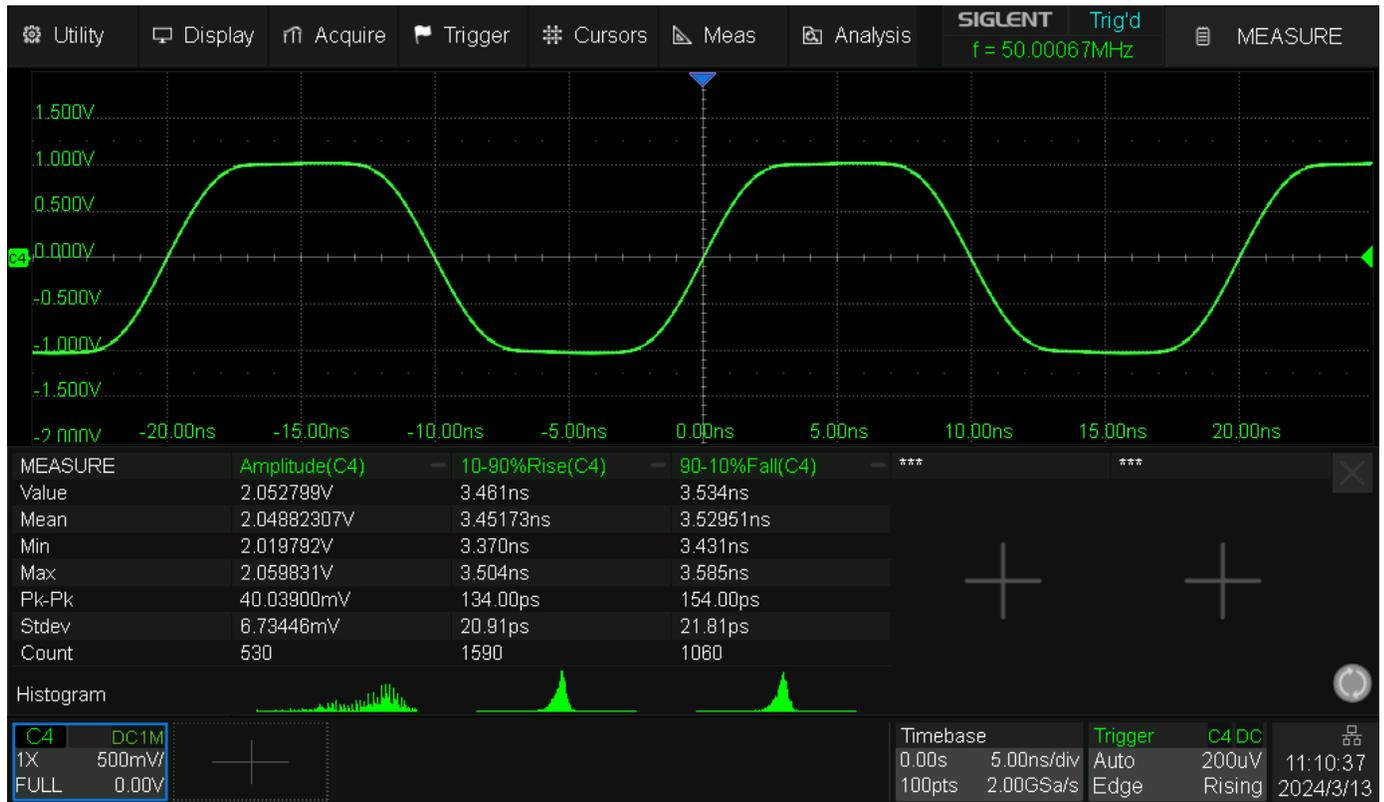
Fig. 186 SDS824X HD\_Square\_3.5ns\_50MHz
