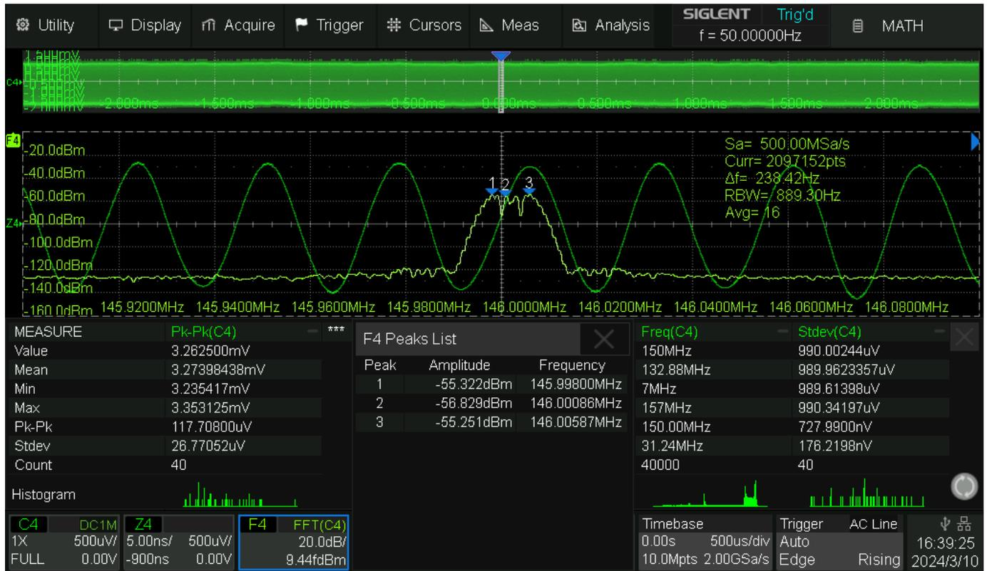
Fig. 176 SDS824X HD\_SA\_FM\_146MHz\_1mV
