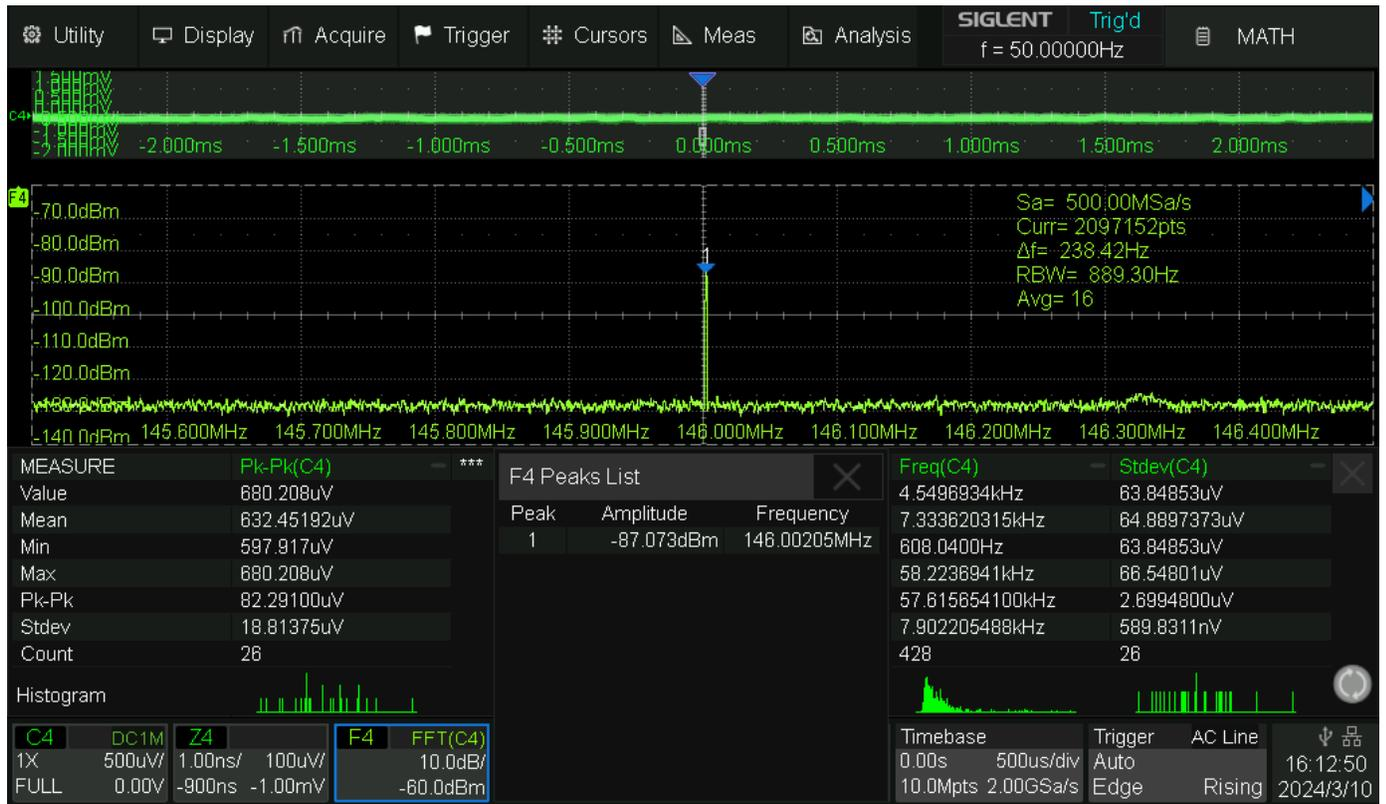
Fig. 173 SDS824X HD\_SA\_CW\_146MHz\_10uV
