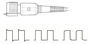
Over-compensated, correct, and under-compensated waveforms
