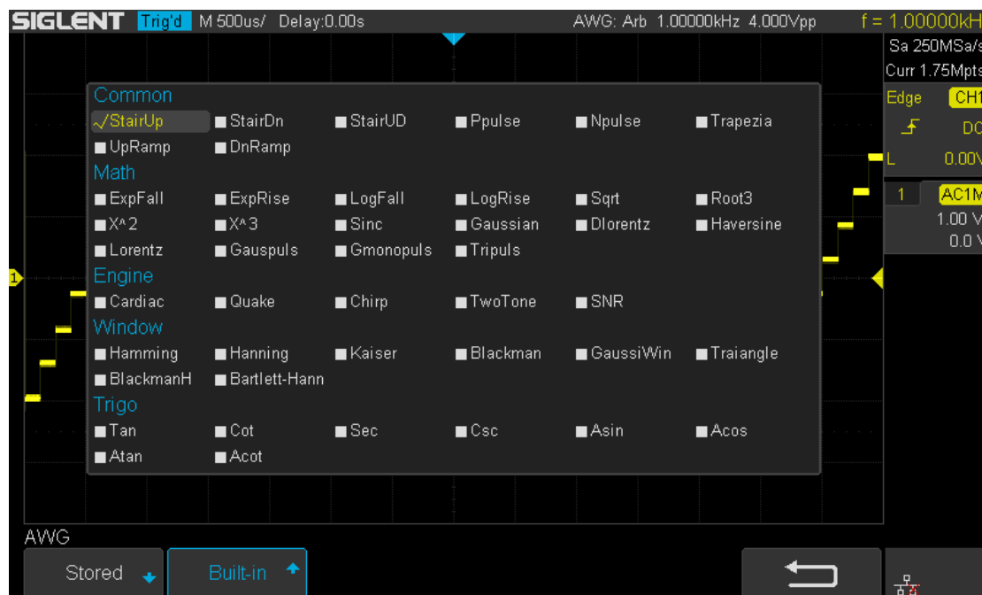
Figure 115 Built-in Arb Interface
