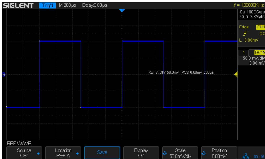
Figure 44 Reference Waveform
