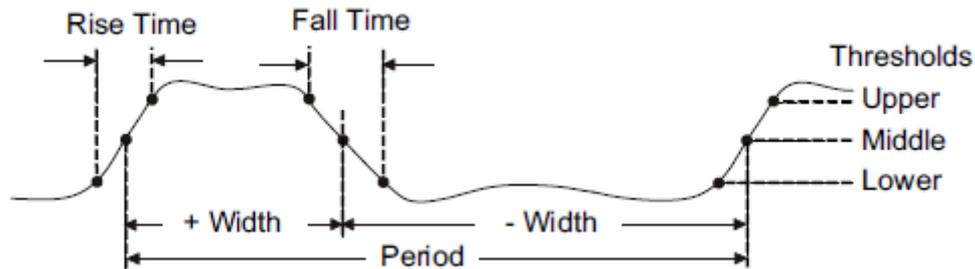
Figure 54 Time Measurements
