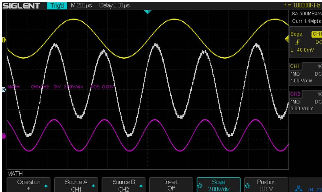
4. If you want to invert the math waveform, press the **Invert** button and set the option to **On** to invert the display of the math waveform.
