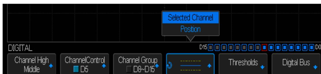
2. Press the fourth softkey to select “**Selected Channel**” and push down the **Universal Knob** to confirm. Turn the **Universal Knob** to select the channel to reposition. The selected waveform is highlighted in red.
