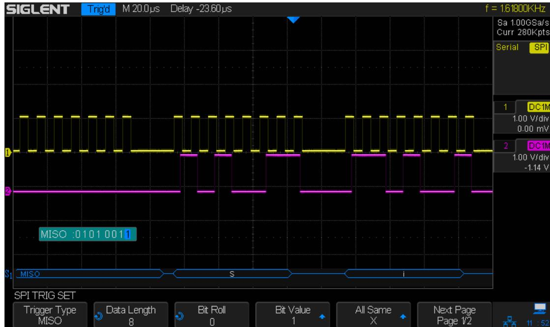
Figure 48 SPI Trigger
