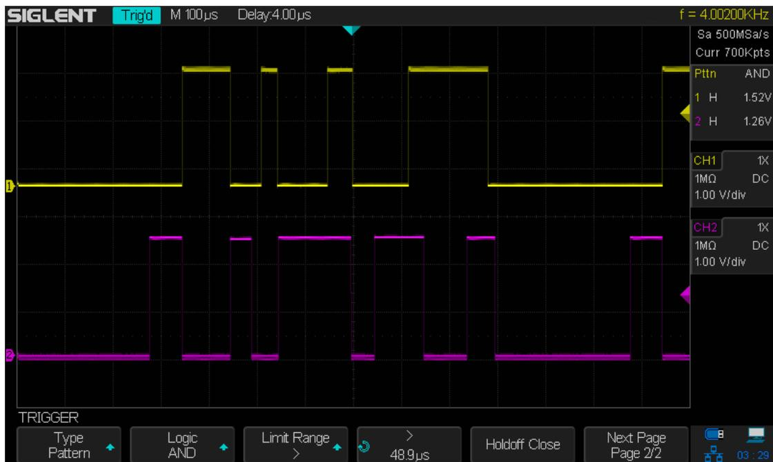
Figure 33 Pattern Trigger
