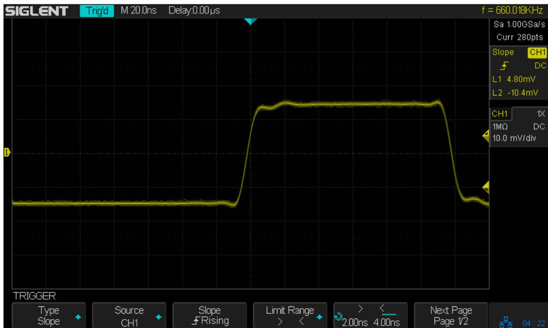
Figure 24 Slope Trigger
