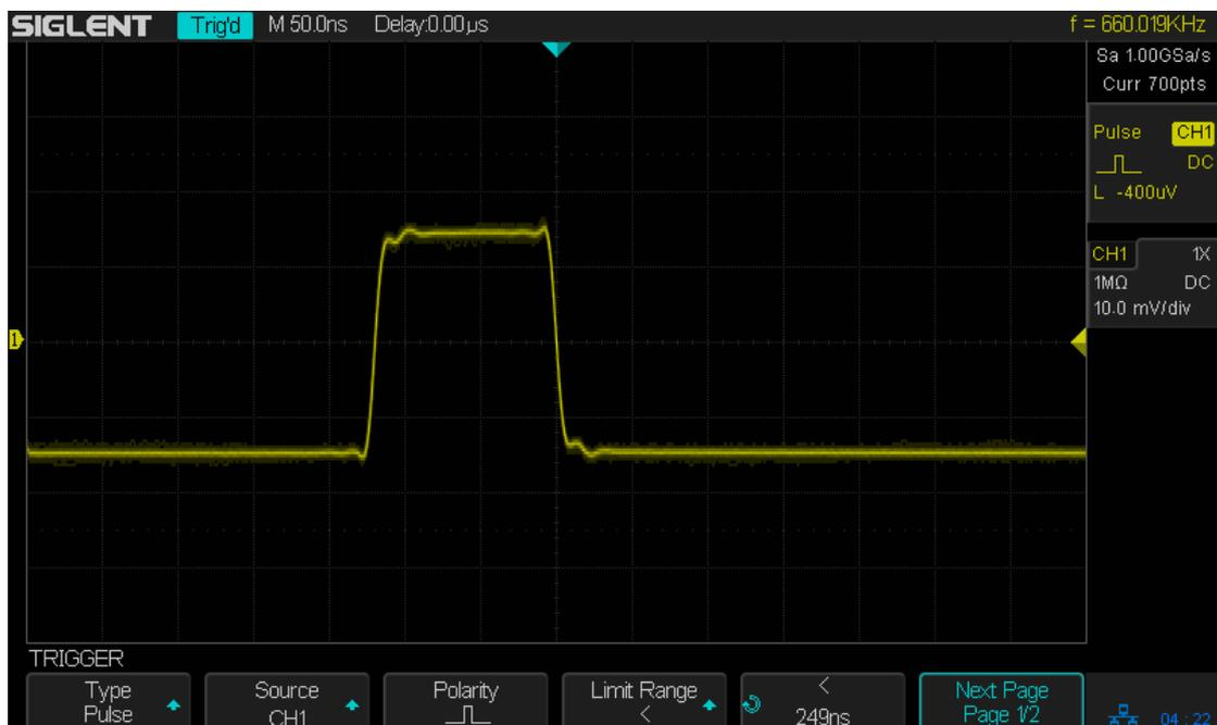
Figure 25 Pulse Trigger
