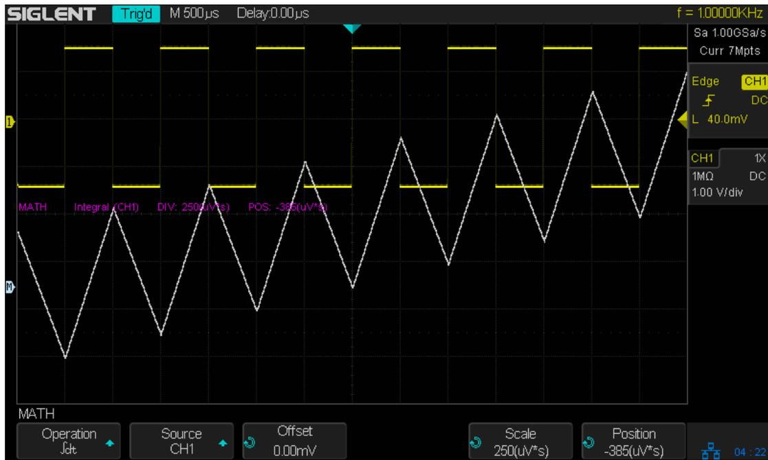
Figure 48 Integral with Offset
