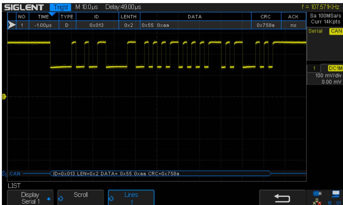
Figure 57 CAN Decode
