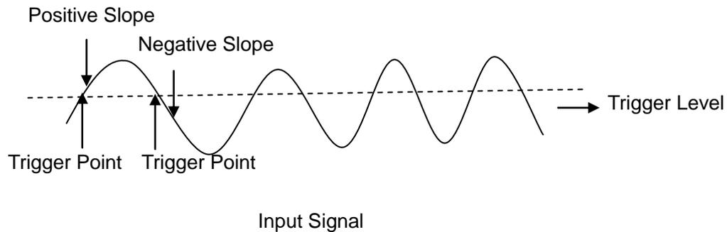
You can adjust the trigger level for a selected analog channel by turning the **Trigger Level Knob**.
