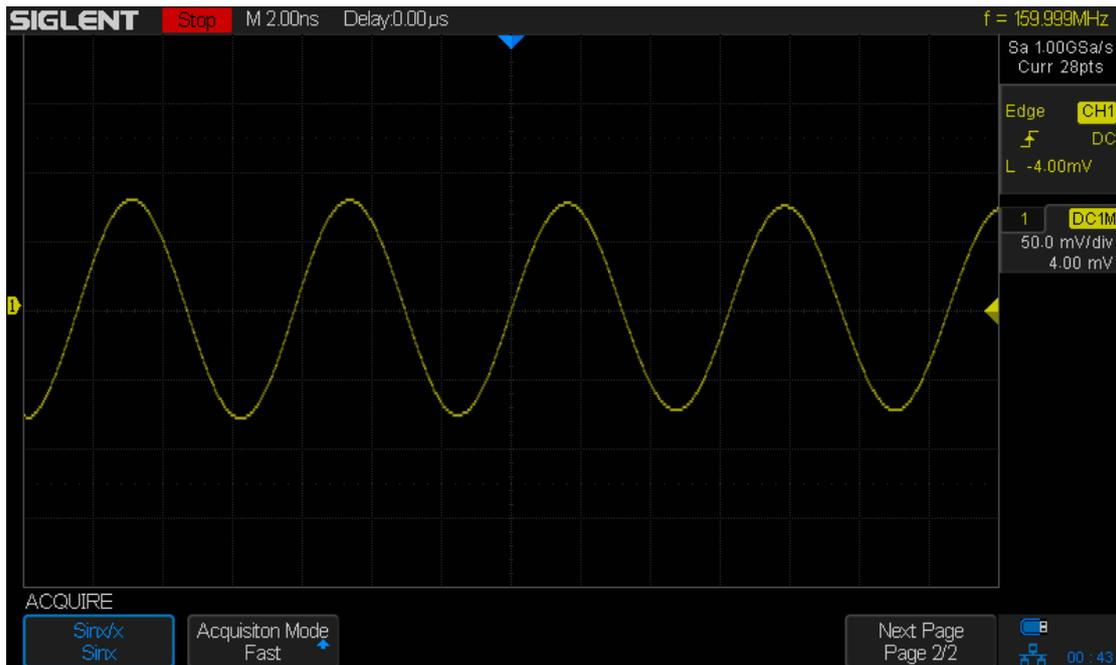
Figure 13 Sinx Interpolation
