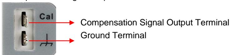
3. Use the probe to connect the input terminal of CH1 of the oscilloscope and the “Compensation Signal Output Terminal” of the probe.
