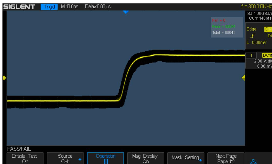
Figure 70 Pass/Fail Test
