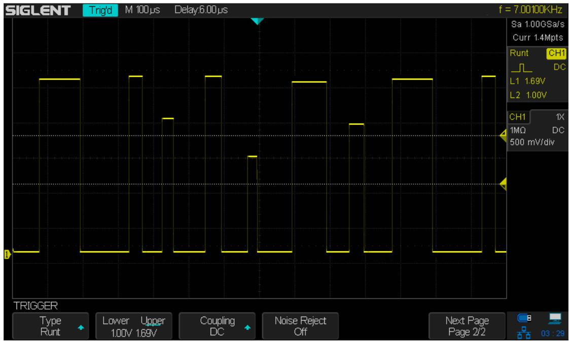
Figure 32 Runt Trigger
