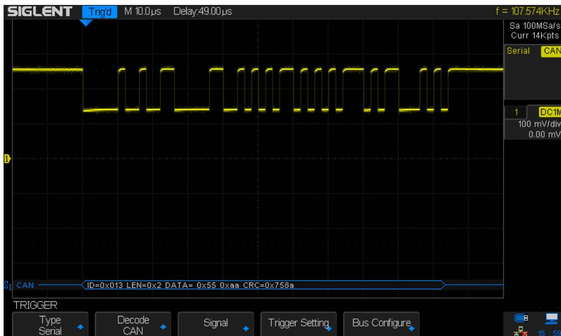
Figure 56 CAN Trigger
